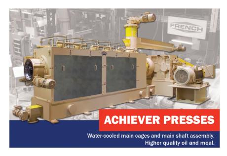
French Achiever presses offer outstanding features and reliability for full pressing to produce full press cake and crude oil. The press design yields high quality oil and cake with residual oils among the lowest in the industry when using the single pressing process. The Model 44, 55, and 66 presses can also be supplied for prepressing oilseeds to produce prepress cake prior to solvent extraction.
