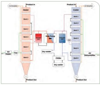
technology – and then cool the product after the RF stage to an ambient temperature for safe handling and storage. Also essential was the ability to recover energy from the hot product at the cooling stage, and then 'upcycle' it for use back at the pre-heating stage.
