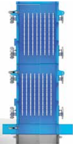
Pic.2 Shifted heat exchange plates
